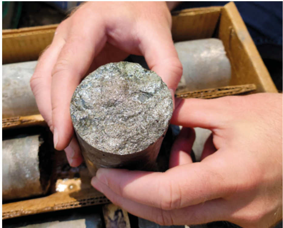
Copper Sulphide in core
