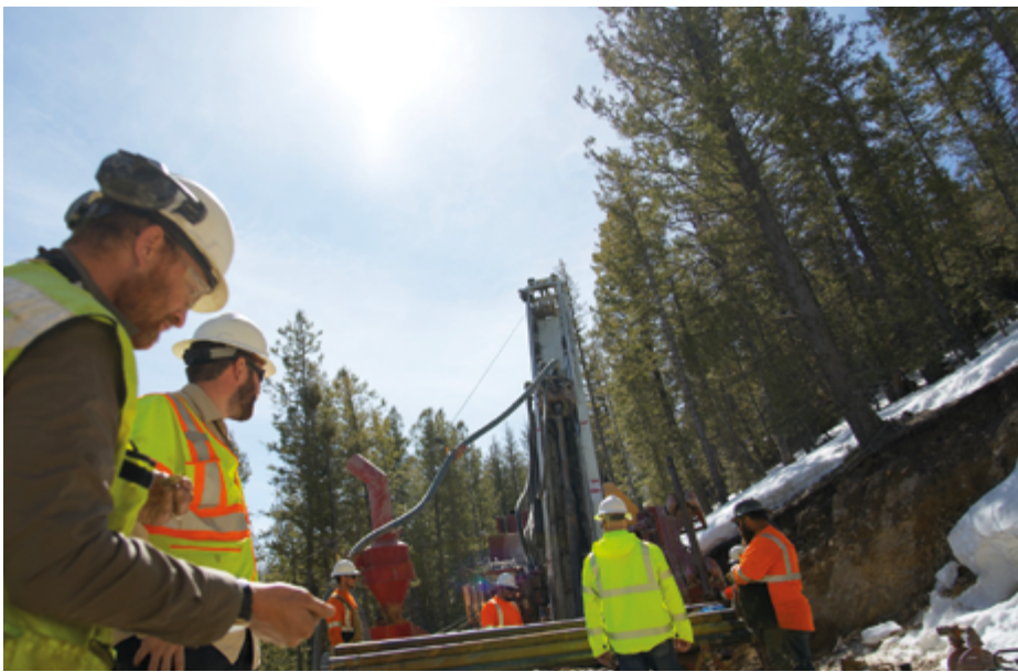
Reverse circulation drilling of Red Star
